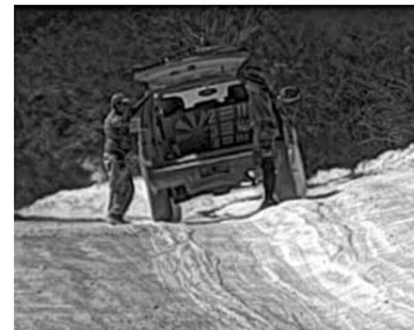
Figure 2. The IVT system processor uses proprietary algorithms to mitigate turbulence-induced blur, apply image stabilization, and enhance contrast (IR imagery shown).
